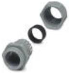
Plastic screw connection up to 5 bar, thread length: 10 mm, cable diameter: 15 - 21 mm, WAF 36, screw connection: M32
