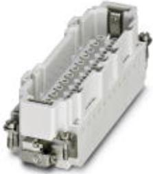
HEAVYCON male insert, B24 series, 24-pos., 25 ... 48 color print, crimp connection. PE connection using tension sleeve technology.
