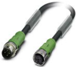
Sensor/actuator cable, 4-position, PUR, black-gray RAL 7021, Plug straight M12 SPEEDCON, coding: A, on Socket straight M12 SPEEDCON, coding: A, cable length: 2 m
