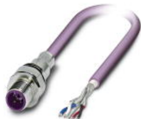
Bus system flush-type plug, DeviceNet/CANopen, 5-pos., M12, shielded, A-coded, front/screw mounting with M16 thread, with 1 m bus cable, 2 x 0.2 mm², 2 x 0.32 mm²
