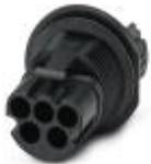
Circular connectors (device-side), Range of articles: PRC, Device connector, rear mounting, housing material: PPE, color: black, number of positions: 5, nom. voltage: 690 V AC, rated current: 35 A, Connection method: Crimp connection, Type of contact: Pin
