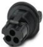
Circular connectors (device-side), Range of articles: PRC, Device connector, rear mounting, housing material: PPE, color: black, number of positions: 3, nom. voltage: 690 V AC, rated current: 35 A, Connection method: Crimp connection, Type of contact: Pin
