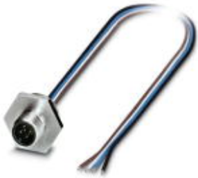
Sensor/actuator flush-type plug, 5-pos., M12, A-coded, front/screw mounting with M20 x 1.5 thread, with 0.5 m TPE litz wire, 5 x 0.34 mm 2 , high-grade steel version
