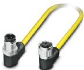
Sensor/actuator cable, 4-position, PVC, yellow, Plug angled M12 SPEEDCON, coding: A, on Socket angled M12 SPEEDCON, coding: A, cable length: 3 m
