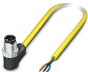
Sensor/actuator cable, 3-position, PVC, yellow, Plug angled M12 SPEEDCON, coding: A, on free cable end, cable length: 2 m
