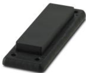
Cable feed-through plates, no. of conductors: 10, length: 154 mm, width: 56 mm, height: 20 mm, external cable diameter: 6x 2 mm ... 8 mm , color: black
