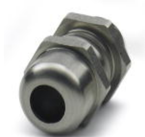
Cable gland, cable gland material: Stainless steel 1.4305, external cable diameter 3 mm ... 6.5 mm, shielding: no, connecting thread: M12 x 1.5, color: silver, with O-ring
