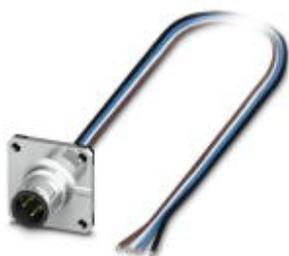
Sensor/Actuator flush-type plug, 4-pos., M12, A-coded, front/square flange mounting, with 0.5 m TPE litz wire, 4 x 0.34 mm<sup>2</sup>
