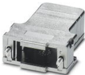
D-SUB sleeve housings, degree of protection: IP20, material: ABS, metal-plated, cable outlet: straight, size of housing: 2, color: Bare metallic
