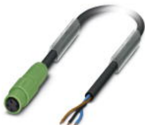
Sensor/actuator cable, 3-position, PUR halogen-free, black-gray RAL 7021, free cable end, on Socket straight M8 Snap-in, cable length: 3 m, with ferrules
