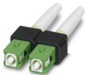
SC duplex connector, with long bend protection, for single mode 9/125 µm, APC polishing (8°), green
