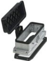
HEAVYCON B24 panel mounting base, for double locking latch, with plastic protective cover, with flat gasket, salt-water-resistant aluminum, conductive profile gasket
