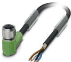
Sensor/actuator cable, 4-position, PUR halogen-free, black-gray RAL 7021, shielded, free cable end, on Socket angled M12 SPEEDCON, coding: A, cable length: 1.5 m
