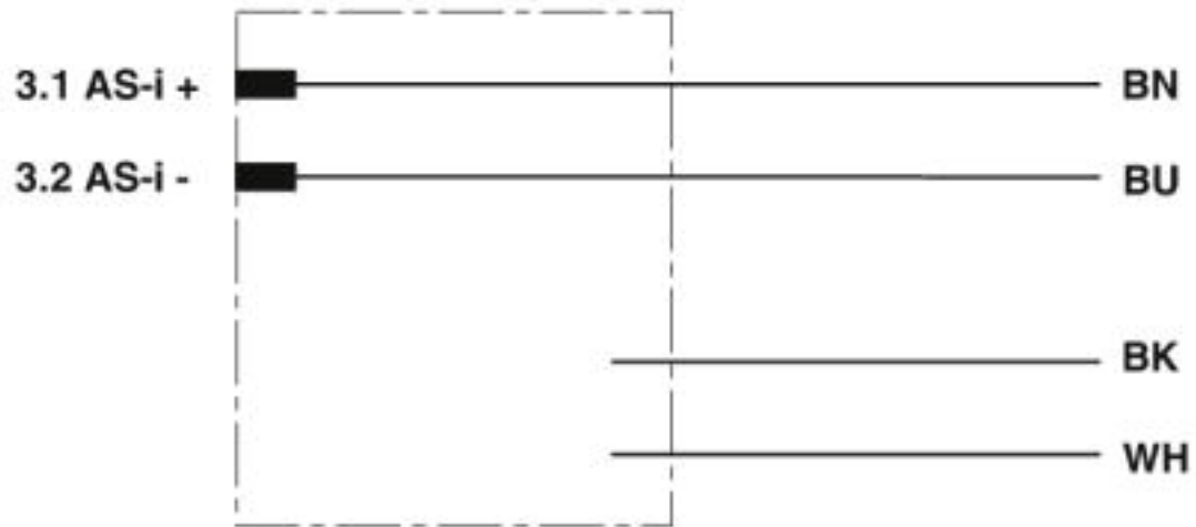
Contact assignment of the AS-Interface distributor
