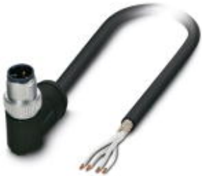
Sensor/actuator cable, 4-position, PE-X halogen-free, black, shielded, Plug angled M12 SPEEDCON, coding: A, on free cable end, cable length: 10 m, For railway applications
