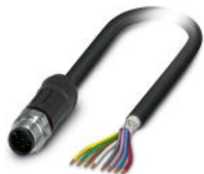
Sensor/actuator cable, 8-position, PE-X/PE-X halogen-free, black-gray RAL 7021, shielded, Plug straight M12, coding: A, on free cable end, cable length: 5 m, for outdoor applications, with high-grade steel knurl
