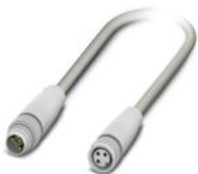
Sensor/actuator cable, 3-position, PP-EPDM halogen-free, gray RAL 7035, Plug straight M8, on Socket straight M8, cable length: 0.3 m, Hygienic design, with plastic knurl
