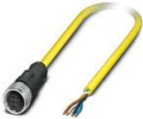
Sensor/actuator cable, 4-position, PVC, yellow, free cable end, on Socket straight M12 SPEEDCON, coding: A, cable length: 10 m
