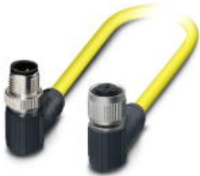
Sensor/actuator cable, 4-position, PVC, yellow, shielded, Plug angled M12 SPEEDCON, coding: A, on Socket angled M12 SPEEDCON, coding: A, cable length: 1.5 m
