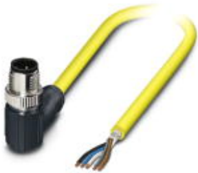
Sensor/actuator cable, 5-position, PVC, yellow, shielded, Plug angled M12 SPEEDCON, coding: A, on free cable end, cable length: 10 m
