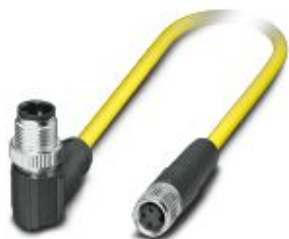
Sensor/actuator cable, 3-position, PVC, yellow, shielded, Plug angled M12 SPEEDCON, coding: A, on Socket straight M8, cable length: 1.5 m
