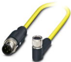
Sensor/actuator cable, 4-position, PVC, yellow, shielded, Plug straight M12 SPEEDCON, coding: A, on Socket angled M8, cable length: 0.5 m
