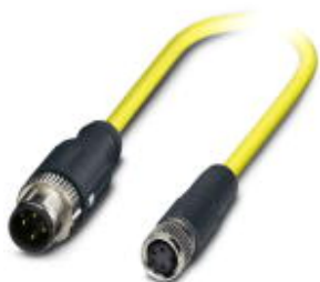
Sensor/actuator cable, 4-position, PVC, yellow, shielded, Plug straight M12 SPEEDCON, coding: A, on Socket straight M8, cable length: 0.5 m
