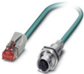
Assembled Ethernet cable, CAT5e, shielded, 2-pair, 26 AWG stranded (7-wire), RAL 5021 (water blue), M12 flush-type socket, rear/screw mounting with SPEEDCON to RJ45 plug/IP20, line, length 0.5 m
