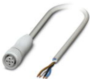
Sensor/Actuator cable, 4-position, PP-EPDM halogen-free, Gray RAL 7035, free cable end, on Socket straight M12, A-coded, Cable length: 5 m, Hygienic design, with plastic knurl
