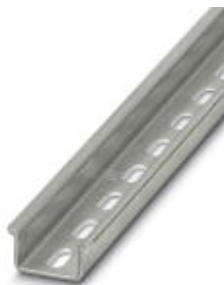
DIN rail perforated, Standard profile, width: 35 mm, height: 15 mm, similar to EN 60715, material: Steel, uncoated, length: 2000 mm, color: white aluminum
