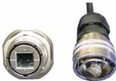
RJF allows you to use an Ethernet Class D / Cat. 5e connection for 10 BaseT, 100 BaseTX or 1000 BaseT networks in harsh environments. With the patented RJStop® system you can use a standard RJ45 cordset in a **metallic** plug which will protect it from shocks, dust and fluids. **No hazardous on-field cabling and grounding!**
