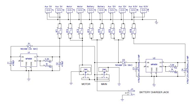
The Arlo Power Distribution Board's charging jack is a convenient way to charge your robot's 12V sealed lead acid batteries without having to disconnect any wiring in your circuits. You can use Parallax's Arlo Smart charger (#700-00245), or another of your own choosing. The charger must be designed for charging Sealed Lead Acid batteries. The input power jack's pin is "center-positive", and is 2.1mm in diameter.
