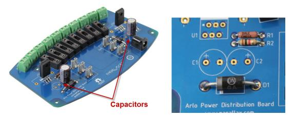
The capacitor's negative terminal will show a (-) sign on the side of its case.
