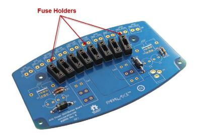
All of the fuse holders should be tight to the board when they're properly soldered.
