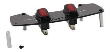
Now, being gentle yet firm, carefully line up the switch connections with the terminals on the PCB and gently "wiggle" the assemblies together such that the standoffs are flat to the PCB.
