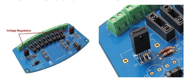
The two voltage regulators are identical, so either can be placed in their respective holes. The regulators are "programmed" to output the required voltages based on the values of each of the resistor pairs (R1, R2), and (R3-R4). For this reason, you must be certain you have installed your resistors correctly.
