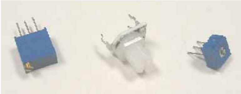
Figure 5-2 A Few Potentiometer Examples
