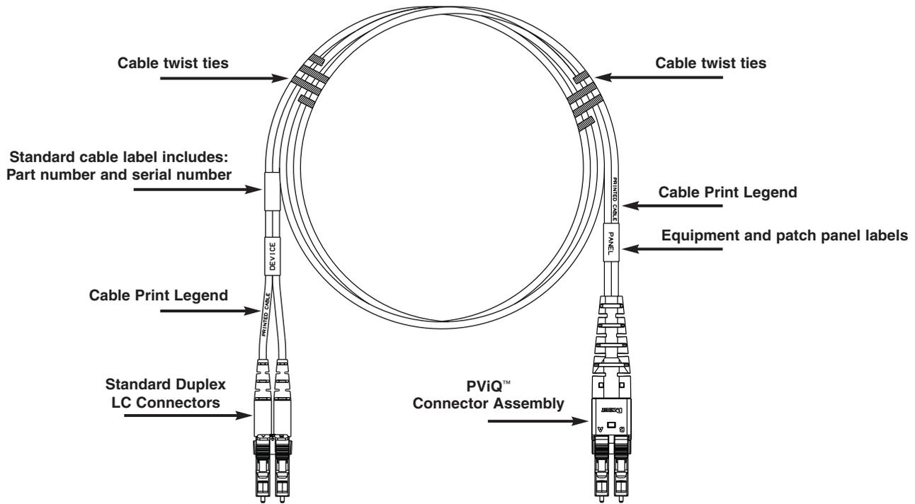
**Example Description: PVQ9LE10LQM05.0** = PanView™ Interconnect Fibre Patch Cord, 9/125µm singlemode, LSZH 1.6mm jacketed, standard duplex LC – to – PanView™ Duplex LC, 5.0 metres long
