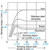
As the sensing object size becomes smaller than the standard size (iron sheet  $10 \times 10 \times t$  1 mm  $0.394 \times 0.394 \times t$  0.039 in), the sensing range shortens as shown in the left figure.
