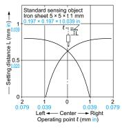
The graph on the left is plotted with the sensitivity adjusted so as to just detect a  $5 \times 5 \times t$  1 mm  $0.197 \times 0.197 \times t$  0.039 in iron sheet placed at a distance of 0.8 mm 0.031 in.
