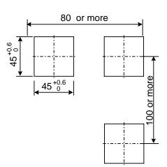
When mounting units in a row Units can be mounted horizontally in a row. In that case, however, waterproofing property on the unit will be lost.
