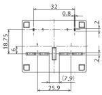
TOLERANCE; less than 10mm:  $\pm 0.3$  min.10mm $\sim$  :  $\pm 0.5$
