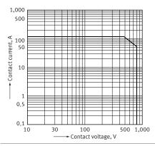
1-2.Max. switching capacity (DC resistive load)
