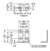
Material: Cold rolled carbon steel (SPCC) Two M4 (length 15mm) screws with washers are attached.
