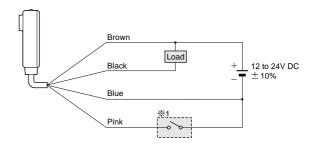
Non-voltage contact, NPN open-collector transistor or NPN non-contact transistor
