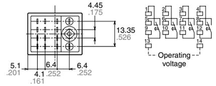
\* For the DC operating type, terminal 14 is "+" and terminal 13 is "-".
