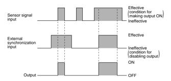
Note: Since NPS-C7 is not incorporated with the selection switch, the output is disabled only when the external synchronization input is Low.
