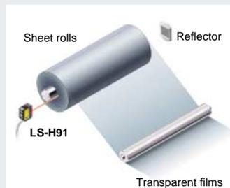
This is a coaxial retroreflective sensor with a spot diameter of approx. φ 1 mm φ 0.039 in (at a 1 m 3.281 ft sensing range), so it can measure amounts remaining on sheet rolls with high precision.
