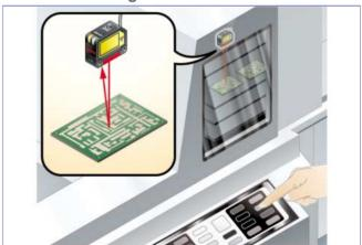
Teaching can be conveniently performed externally for laser sensors installed inside a device.
