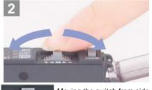
Moving the switch from side to side allows items to be selected
