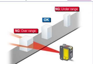
The sensor judges any object outside the range of incident light intensity established by two set threshold values.
