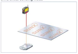
Only rapid changes in light received are detected, which enable the edge of glass, etc. to be detected accurately. Optimal for positioning.
