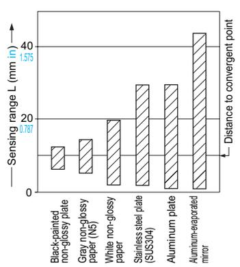
The bars in the graph indicate the sensing range (typical) for the respective material. However, there is a slight variation in the sensing range depending on the product. Further, if there is a reflective object (conveyor, etc.) in the background of the sensing object, since it affects the sensing, separate it by more than twice the sensing range shown in the left graph, or adjust the sensitivity adjuster.
