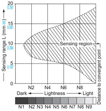
The sensing region (typical) is represented by oblique lines in the left figure. However, the sensitivity should be set with enough margin because of slight variation in products.
