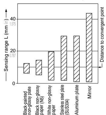
The bars in the graph indicate the sensing range for the respective material. However, there is a slight variation in the sensing range depending on the product. Further, if there is a reflective object (conveyor, etc.) in the background of the sensing object, since it affects the sensing, separate it by more than twice the sensing range shown in the left graph, or adjust the sensitivity adjuster.
