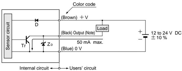
Note: The emitter of the thru-beam type sensor does not incorporate the output.
