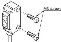
Note: When mounting the front sensing type sensor, use M3 pan head screws without washers, etc.
