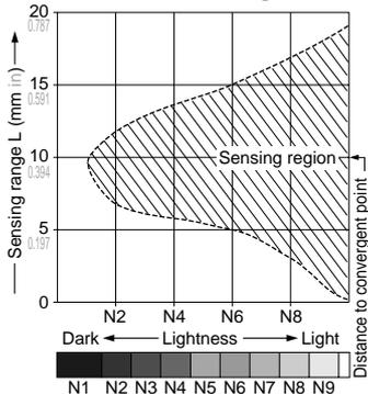
The sensing region is represented by oblique lines in the left figure. However, the sensitivity should be set with enough margin because of slight variation in products.
