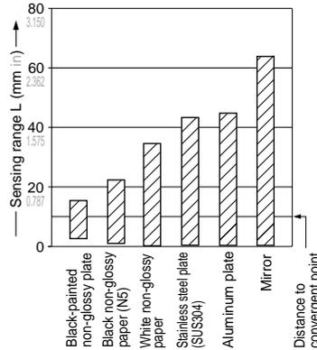
The bars in the graph indicate the sensing range for the respective material. However, there is a slight variation in the sensing range depending on the product. Further, if there is a reflective object (conveyor, etc.) in the background of the sensing object, since it affects the sensing, separate it by more than twice the sensing range shown in the left graph.
