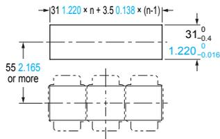
Note: The panel thickness should be 1 to 6 mm 0.039 to 0.236 in.
