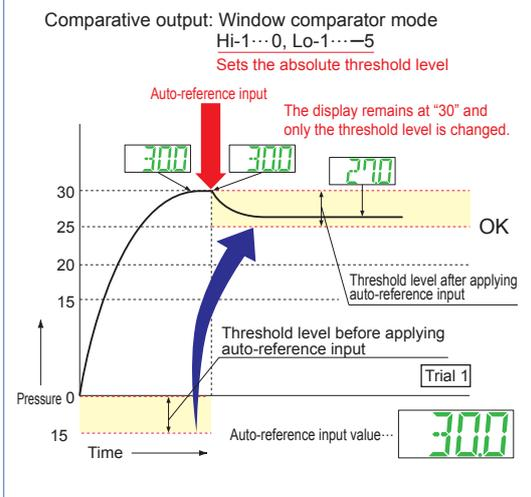
When auto-reference input is applied, the reference pressure "30" is added to the threshold level. If the reference pressure changes to "20" or "40", the auto-reference input compensates for this every time by changing the threshold level, so any variation in the filling pressure can be ignored.
