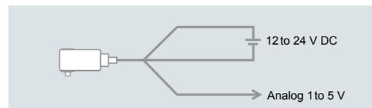
The analog voltage output from the sensor head can be picked up directly.
