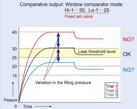
Because the threshold level is fixed for conventional pressure sensors, changes in the reference pressure result in wrong decisions.
