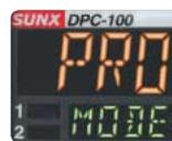
High-level function settings such as hysteresis adjustment and the copy function can be carried out.
