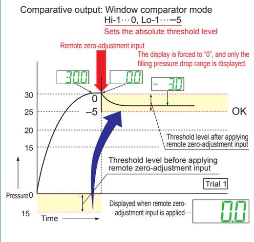
When remote zero-adjustment input is applied, the reference pressure is forced to "0". If the reference pressure changes to "20" or "40", the remote zero-adjustment input adjusts the reference pressure to "0" every time the reference pressure changes, so any variation in the filling pressure can be ignored.
