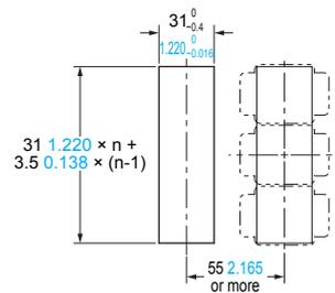
Note: The panel thickness should be 1 to 6 mm 0.039 to 0.236 in.
