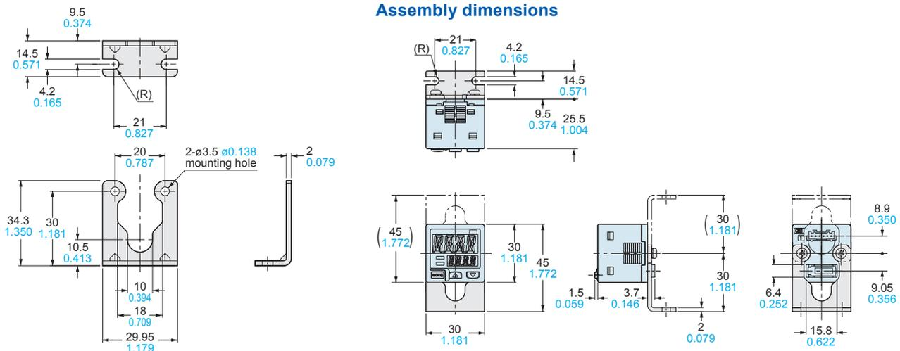
Material : Cold rolled carbon steel (SPCC) (Uni-chrome plated)
