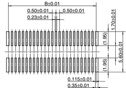
\* See the dimension table on page 102 for more information on the B dimension of the socket and header.
