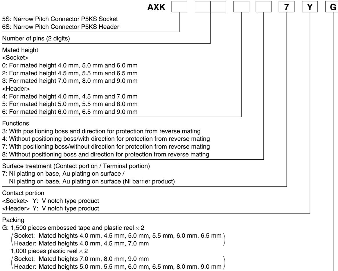
Note: Models with mating directionality to prevent reverse insertion have less than 100 pin contacts. Models without mating directionality to prevent reverse insertion have over 100 pin contacts.
