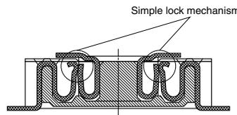
**5. The lower connector bottom surface construction prevents contact and shorts between the PCB and metal terminals.** Benefits include freedom in pattern wiring, helping to make PCB's smaller.
