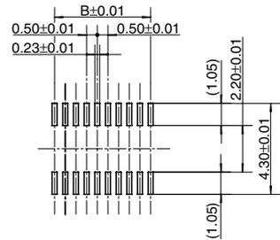
\* See the dimension table on page 4 for more information on the B dimension of the socket and header.
