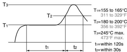
Temperature rise of relay itself may vary according to the mounting level or the heating method of reflow equipment. Therefore, please set the temperature of soldering portion of relay terminal and the top surface of the relay case not to exceed the above mentioned soldering condition.
