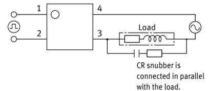
2) When Clamp diode or CR Snubber is used in the circuit, the spike voltages from the load are limited. But the longer wire may become the inductance and cause the spike voltage. Keep the wire as short as possible.
