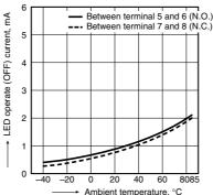
6. LED reverse current vs. ambient temperature characteristics Load voltage: 400 V (DC); Continuous load current: 100 mA (DC)
