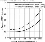
4. Reverse time vs. ambient temperature characteristics
