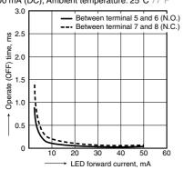
11. Reverse time vs. LED forward current characteristics
