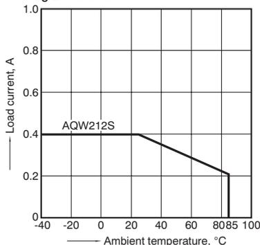
1-(2) Load current vs. ambient temperature characteristics
